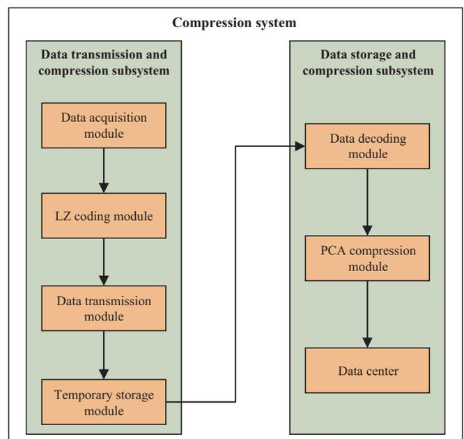
Fig. 4. Compression system for smart meter data to relieve data transmission line burden and reduce storage overhead.
